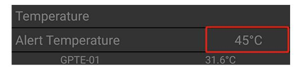
When the internal temperature of the device exceeds the value set by Alert Temperature: the brightness of the device is forcibly reduced to 50%. When the temperature drops by 10°C, the original brightness control will be restored.
