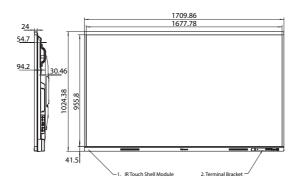
**86"**  $\begin{vmatrix} 1955^{\text{W}} \text{ x } 1162.5^{\text{H}} \text{ x } 126^{\text{D}} \text{ mm} / 77 \text{ x } 45.8 \text{ x } 5 \text{ inch } 58 \text{ kg} / 127.89 \text{ lbs} \end{vmatrix}$
